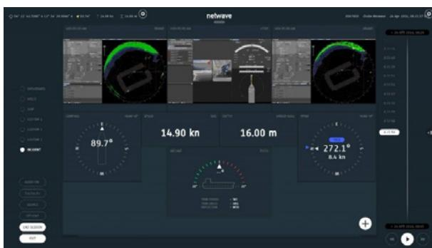
VDRs are data recording systems, mandated for commercial vessels in international waters under MSC. 333(90), to enable accident investigators to review procedures and instructions in the moments before an incident and help to identify the cause of any accident for ocean going vessels.
