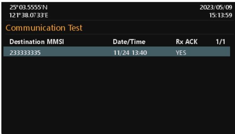
Press **Fn** to start the communication test. The system will show Target List that only has targets with Class A type. Use direction keys to select a target and then press **↑** to start the transmission of Message 10.
