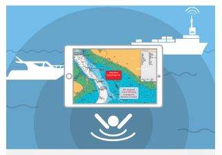
MOB incident results in activation of AIS MOB device, which transmit a localised locating signal on maritime VHF frequencies to a range of 4 miles (approx).
