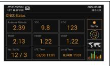
Shows the GNSS satellite current usage status (Refer to section 4.7.4 GNSS Status)
