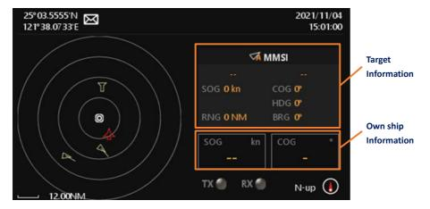
Radar View displays own ship and target ships' statuses, and their correlations. It is a proportional chart scale showing the current ratio displayed. The distance between the inner and outer circles (1 grid) is the number displayed on the scale at left bottom. You can adjust the scale to display ships in different distances.
