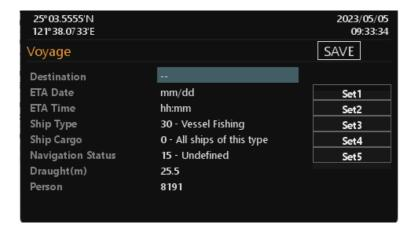
**Notice**: if Ship Type is Tanker, by regulation, whenever the ship navigation status is "Moored", the transponder's transmission power is automatically changed to 1W for safety measures.
