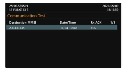
Press to start the communication test. The system will show Target List that only has targets with Class A type. Use direction keys to select a target and then press to start the transmission of Message 10.
