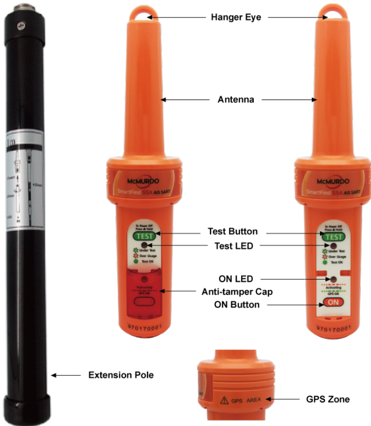
Figure 1: AIS SART key features description
