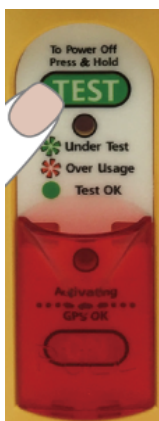
Figure 11: Testing of AIS SART
