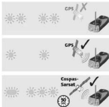
While the PLB is active, pressing the **ON** button again will cause the indicator light to flash a Morse code SOS pattern. This can be used to attract attention in low light conditions. The SOS pattern is repeated four times each time **ON** is pressed.
