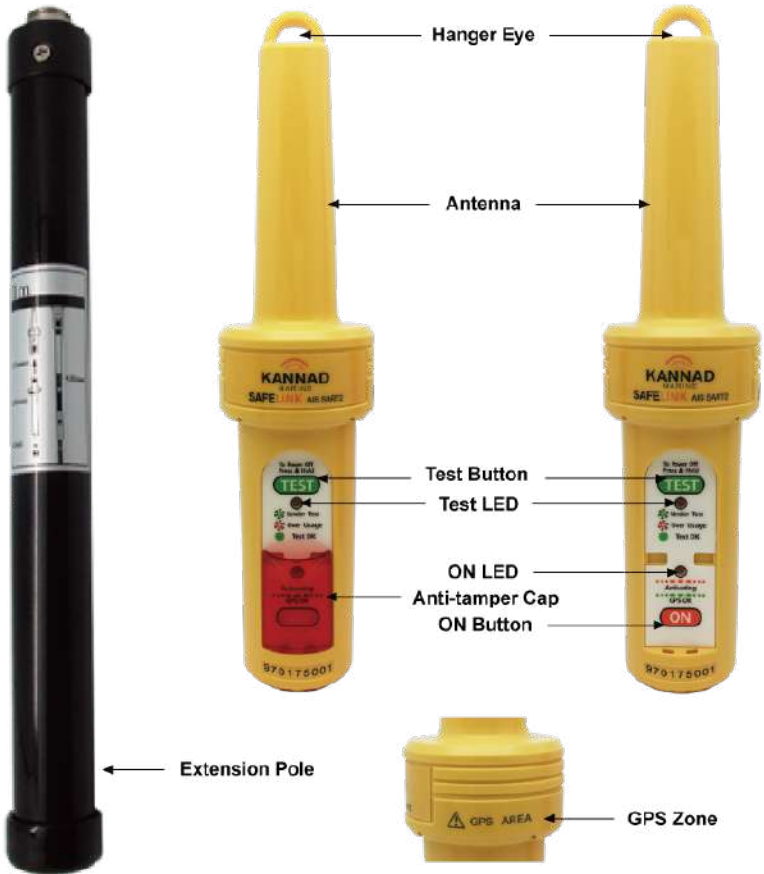
Figure 1: AIS SART key features description
